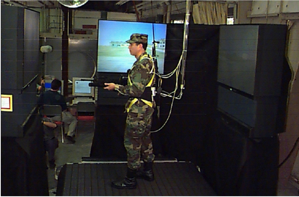
Figure 10. Omni-directional Treadmill (ODT) Photo courtesy of Darken, R. Naval Postgraduate School, Monterey, CA.
