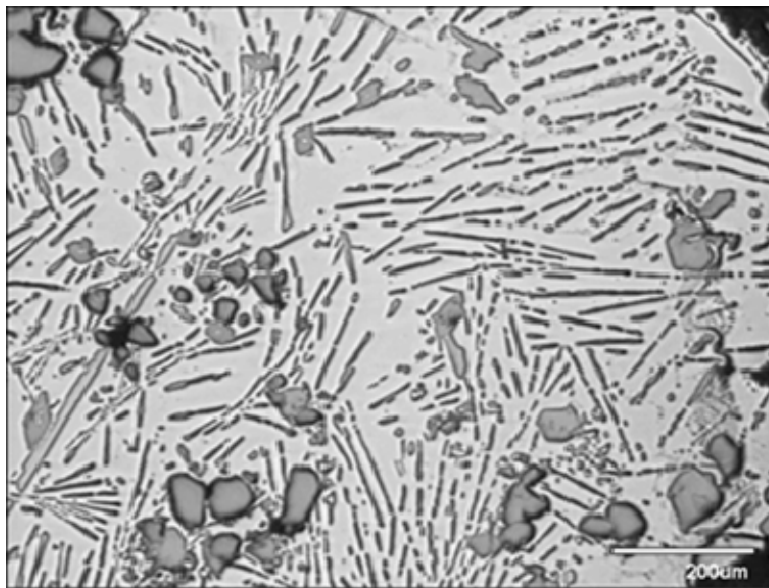
Figure 32. 290x Optical Microscopy NiTi Powder Reinforced Solder.
