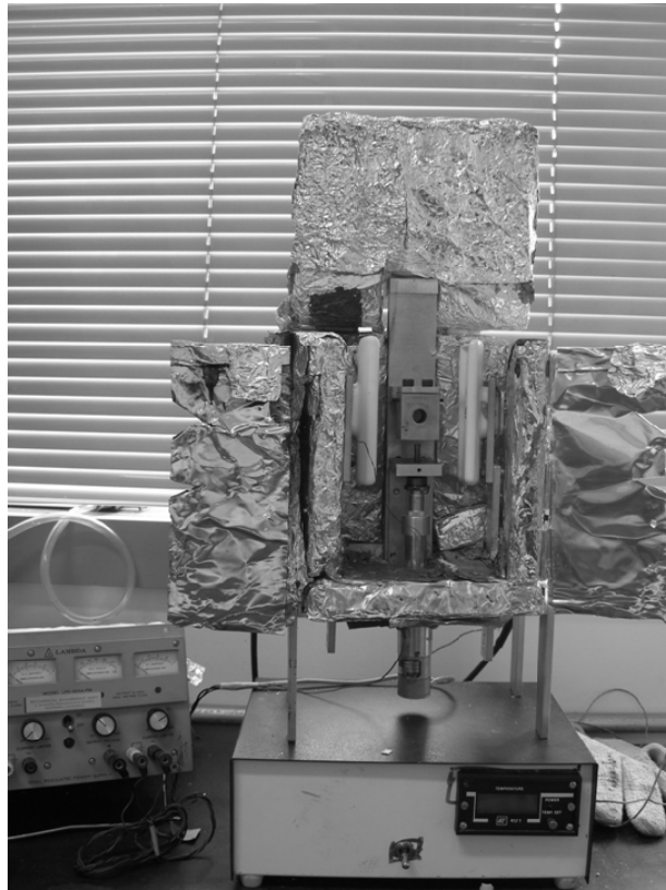
Figure 6. Furnace and Fixture for Manufacture of SJS Type Joint.
