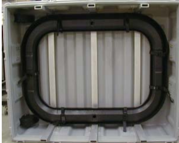
Figure 21. Cable storage in ODU cover
