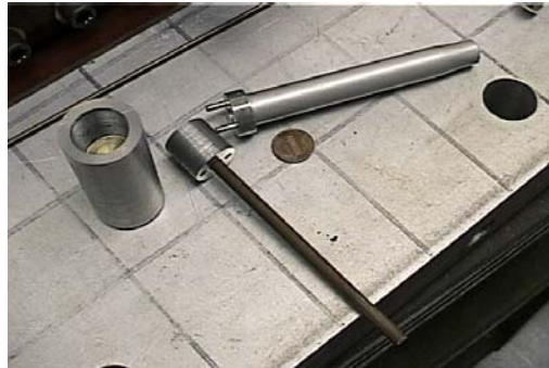
Figure 2.6 Break-down of pusher assembly with rod replacement tool.
