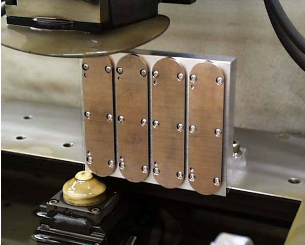
Figure 2.10 EDM set up for groove rail fabrication.
