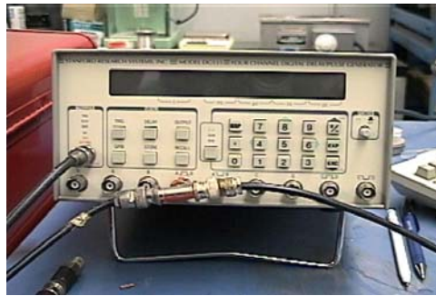
Figure 2.9 Delay generator receives input from OTC and sends firing command signal to rail gun.
