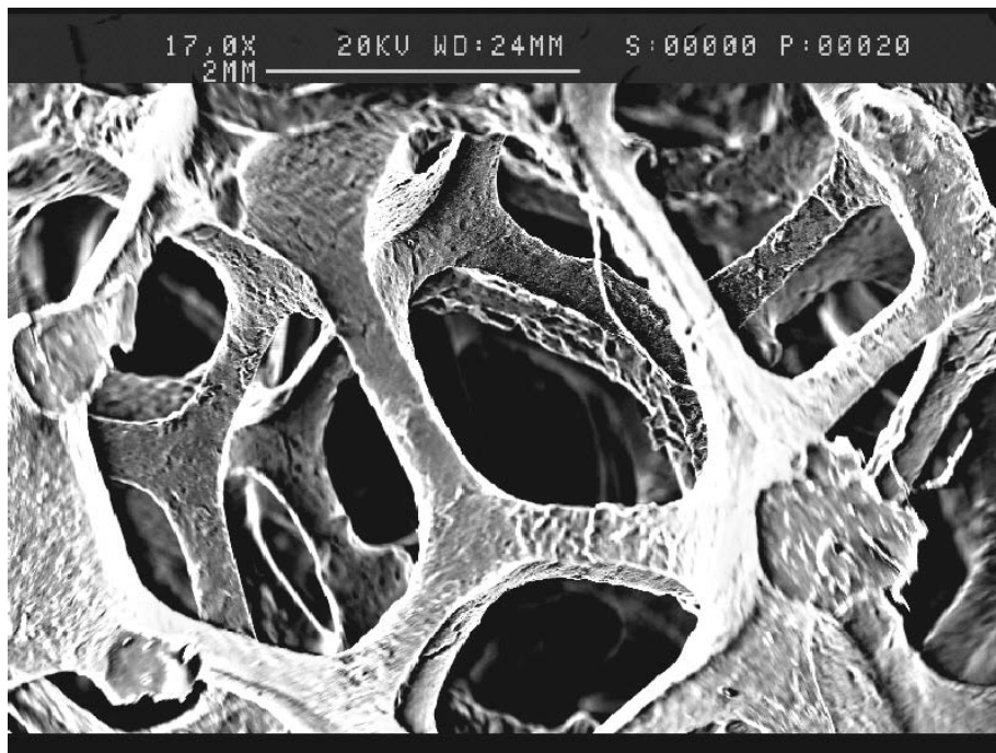
Figure 29 SEM Image of 20 PPI Aluminum Foam Before Compression
