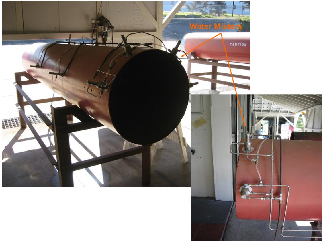
Figure 14. Noise Suppression System
