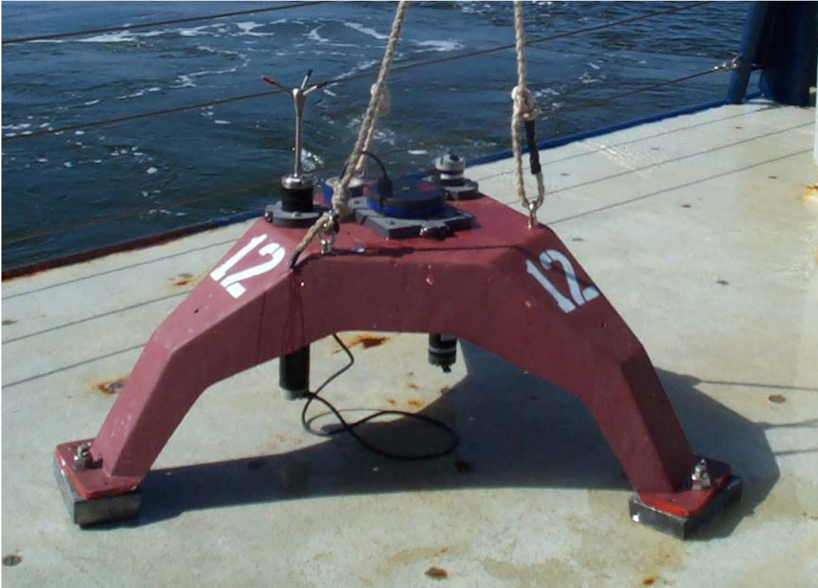
Figure 9. Nortek Vector Current Meter about to be deployed during NCEX. Similar to the pressure sensor, the instrument is mounted in a red fiberglass tripod equipped with lead feet. The three receiver arms of the probe are seen above the left leg of the tripod, while the pressure sensor is located in the center of the instrument. A spare battery is located in the center of the tripod and a Nortek Aquadopp Velocity profiler is mounted near the rear leg.
