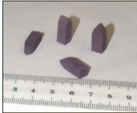
Figure 2.A.5 Lockwood's 1.2-meter railgun projectiles from Ref. [5]
