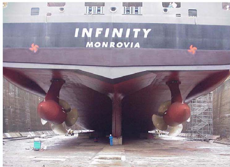
Figure 7.3. Picture showing the mounting of two pulling type pods (From Ref. 30.)
