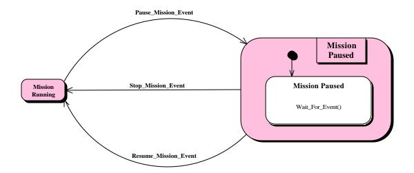
Figure 12. State diagram of the Pause Mission function.
