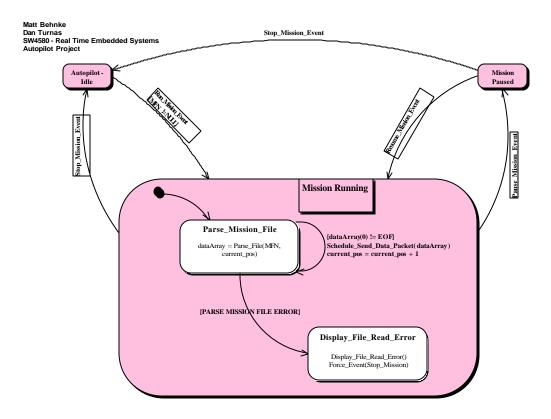
Figure 11. State diagram of the Run Mission function.
