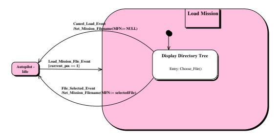
Figure 10. State diagram of the Load Mission function
