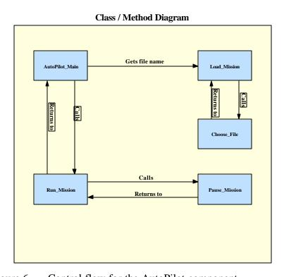
Figure 6. Control flow for the AutoPilot component
