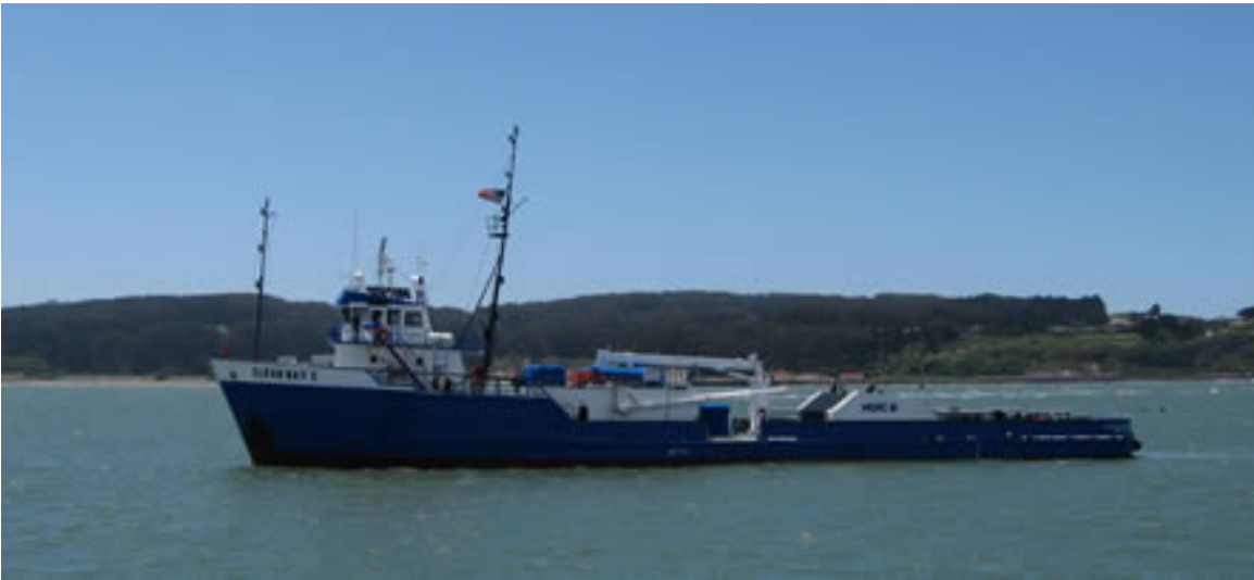
Figure 6. The target vessel Clean Bay II which was used in TNT 07-3 MIO. The “Old Glory” on the mast behind the bridge was a useful feature. Ranges were recorded when the flag was first seen (but no features on it) when the stripes were distinct and when the stars were visible using the naked eye and binoculars. Other features that were observed were the lettering on the bow, the bridge windows, a sign on the side (not seen here, see Figures 8 and 9) and people.
