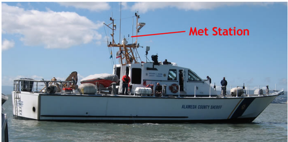
Figure 3. Photograph of the Alameda County Sheriffs Boat (ACSB), the location of the ship met station during the TNT 07-3 MIO. The met station itself does not clearly stand out, but it is possible to see the sonic anemometer just to the left of the red indicator line. This was the same location used in the other FY 2007 TNT MIO programs.
