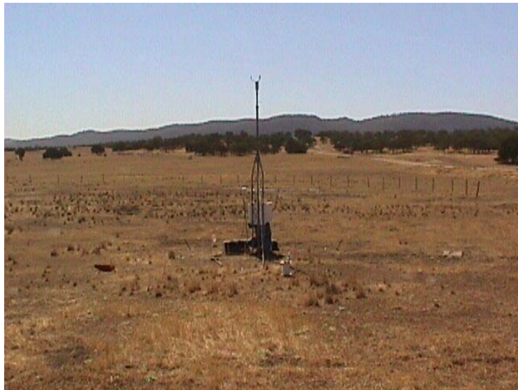
Figure 3. Instrumented portable meteorological (MET) tower installed at McMillan Field. Instrumentation listed in Table I-1 of Appendix I.
