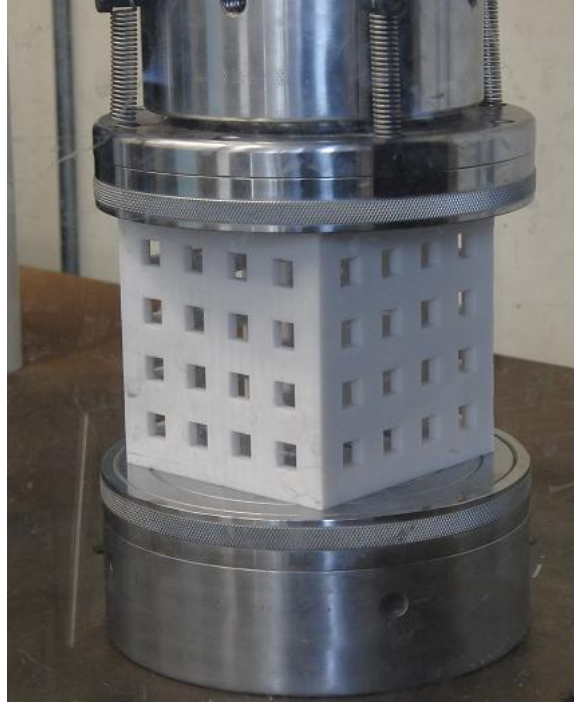
Figure 6. CS2 structure mounted for compression testing.
