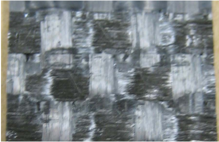
Figure 26. Surface crack propagation path for a co-cured coupon.
