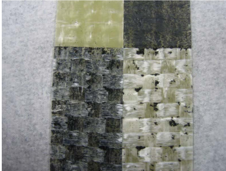
Figure 44. Surface view of crack propagation path in fiberglass coupon with CNTs.
