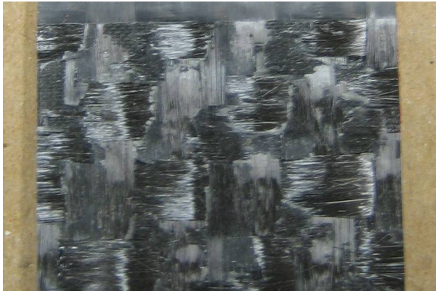
Figure 27. Surface crack propagation path for a two-step cured coupon.
