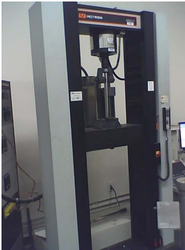
Figure 19. Mode II test setup in Instron test machine.
