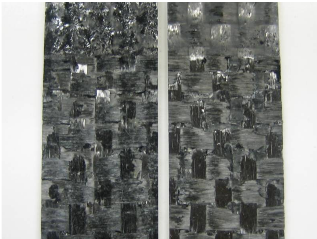
Figure 34. Crack propagation path of carbon fiber composite with CNTs.
