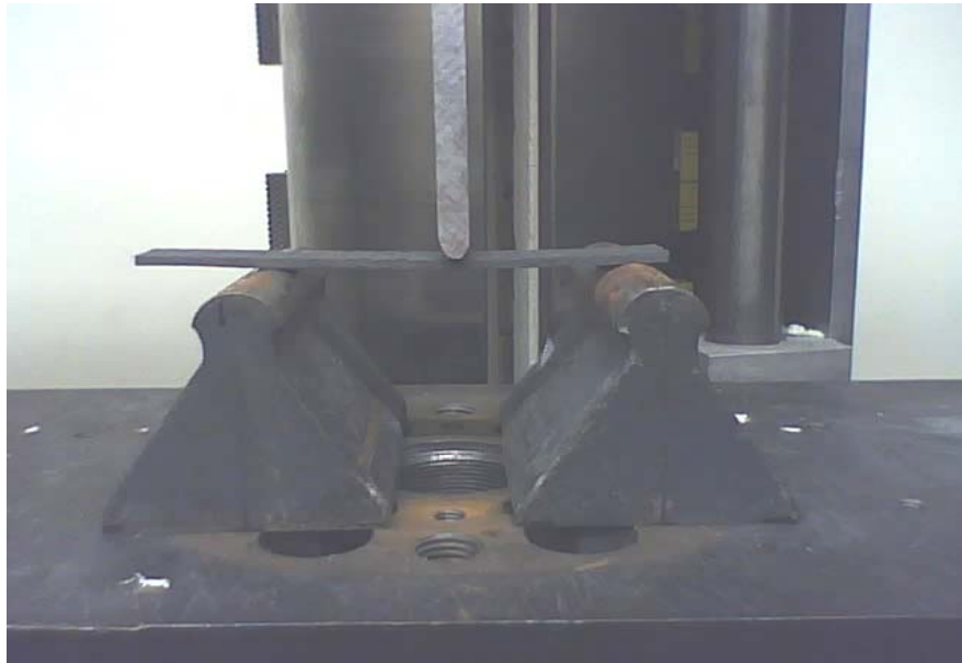
Figure 22. Picture of three-point bending test for Mode II.
