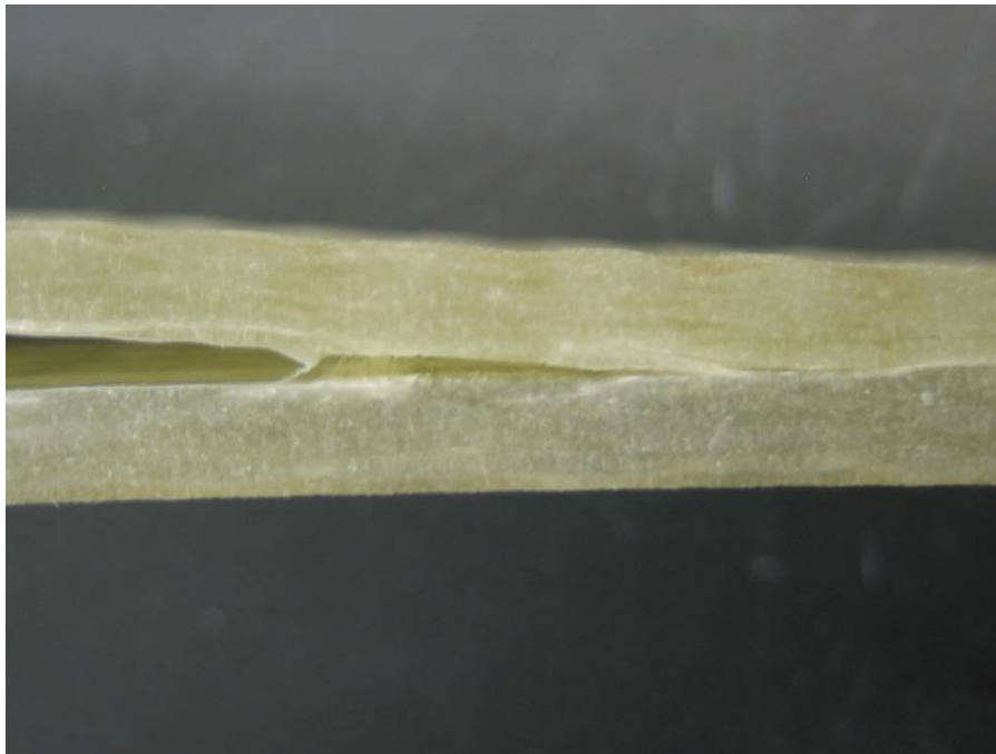
Figure 41. Crack propagation image for fiberglass coupon without CNTs.
