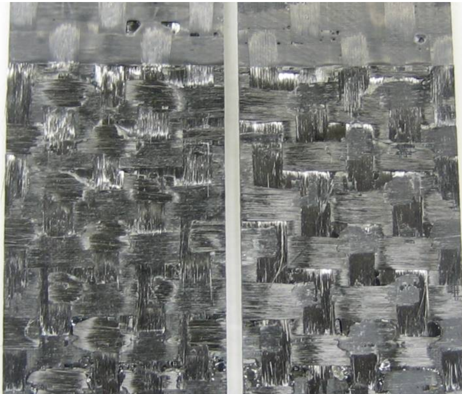
Figure 33. Crack propagation path of carbon fiber composite without CNTs.
