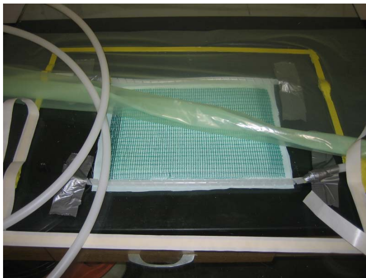
Figure 11. Rolling out the plastic sheet used to form the vacuum bag.
