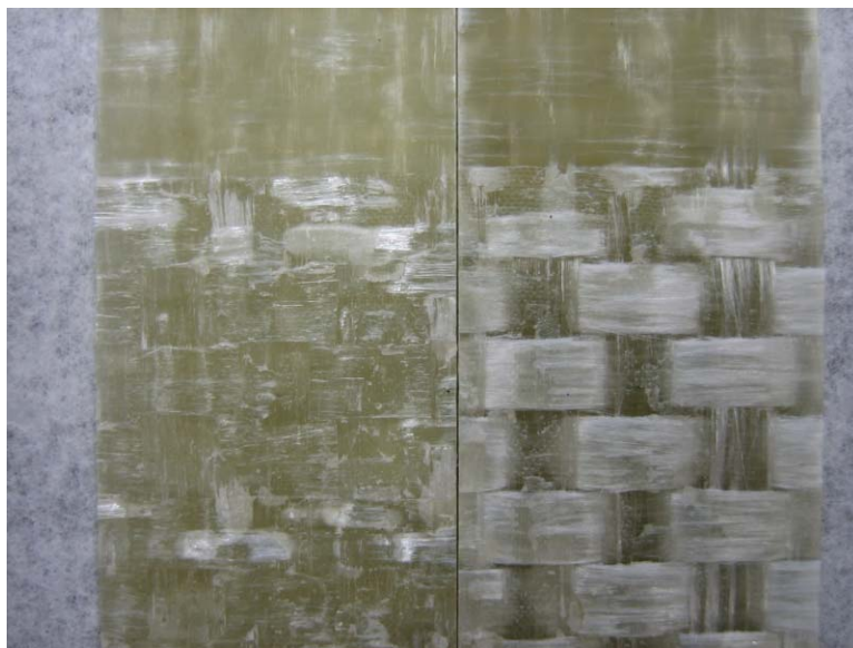
Figure 45. Surface view of crack propagation path in fiberglass coupon without CNTs.
