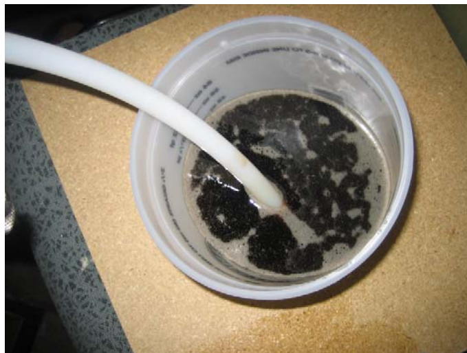
Figure 13. Resin at inlet with bubbles after mixing.
