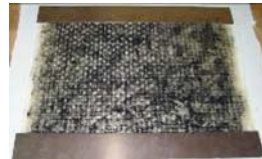
CNTs dispersed on carbon fiber composite interface improved fracture strength while acting as in situ sensor
