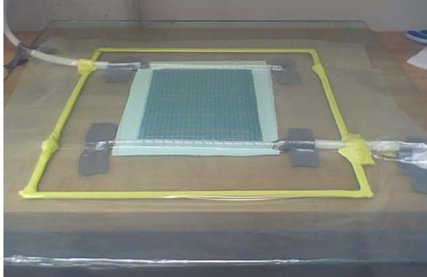
Figure 12. Sample setup under vacuum.
