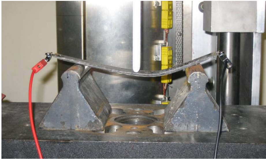
Figure 28. Carbon fiber Mode II resistance testing in bent position.
