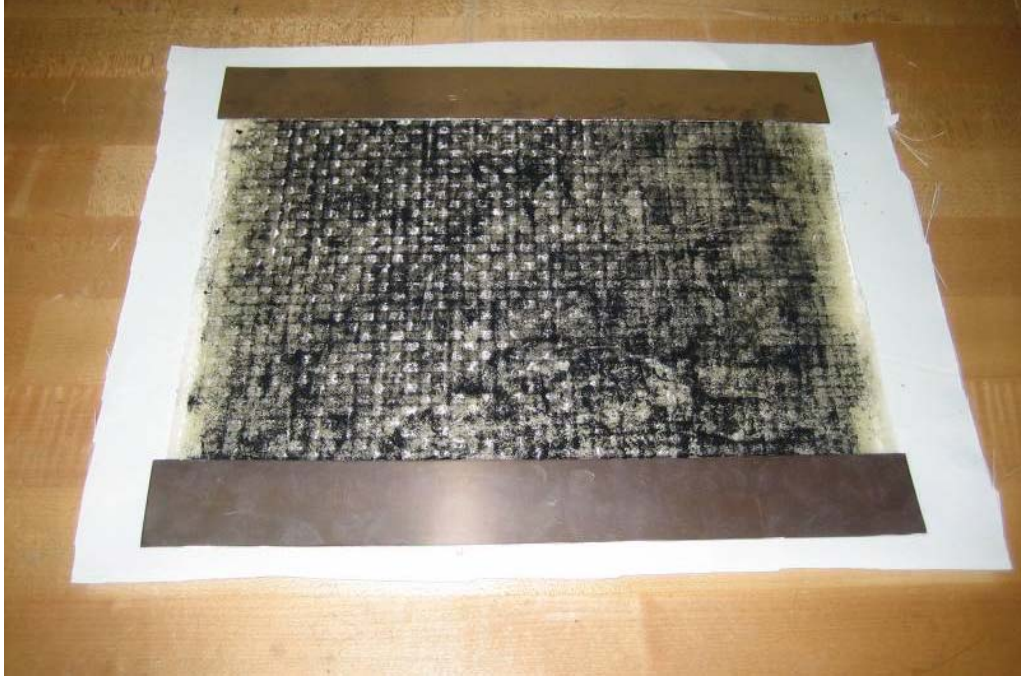
Figure 16. Bottom layer of two-step cured sample covered with CNTs.
