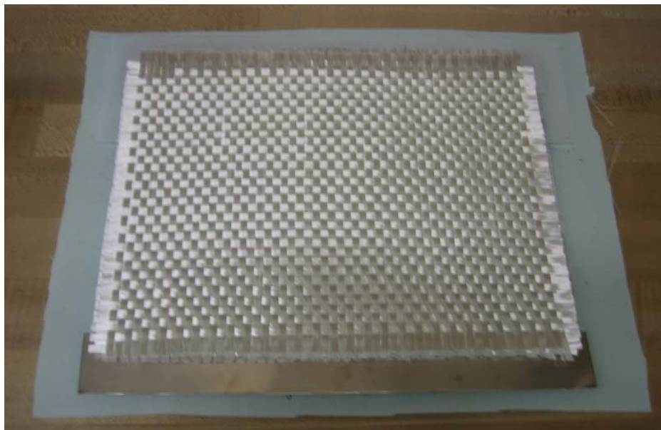
Figure 18. Remaining fiber material stacked on top of bottom plate.
