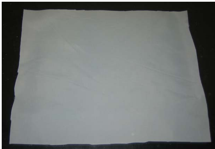
Figure 5. Peel ply laid on top of distribution media for co-cured samples.
