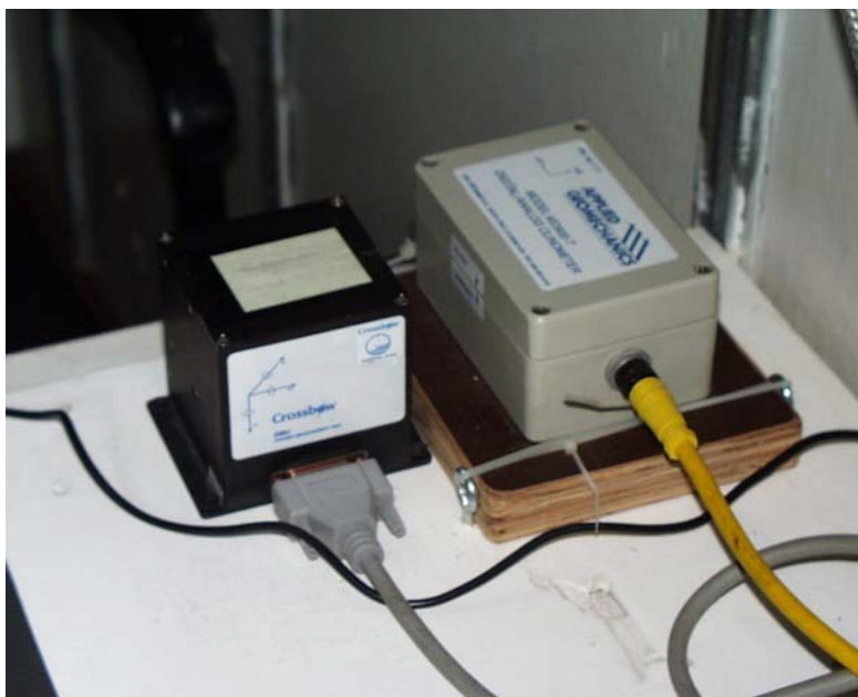
Figure F3. Close-up of the vertical gyro (left) and tiltmeter (right) mounted on a lab bench in the main lab of R/V Point Sur .
