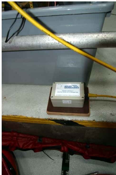
Figure F6. Tiltmeter mounted forward of the moon pool on R/V Western Flyer .
