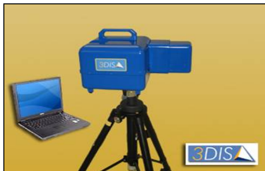
Figure 11. SIS Laser Scanning Equipment
