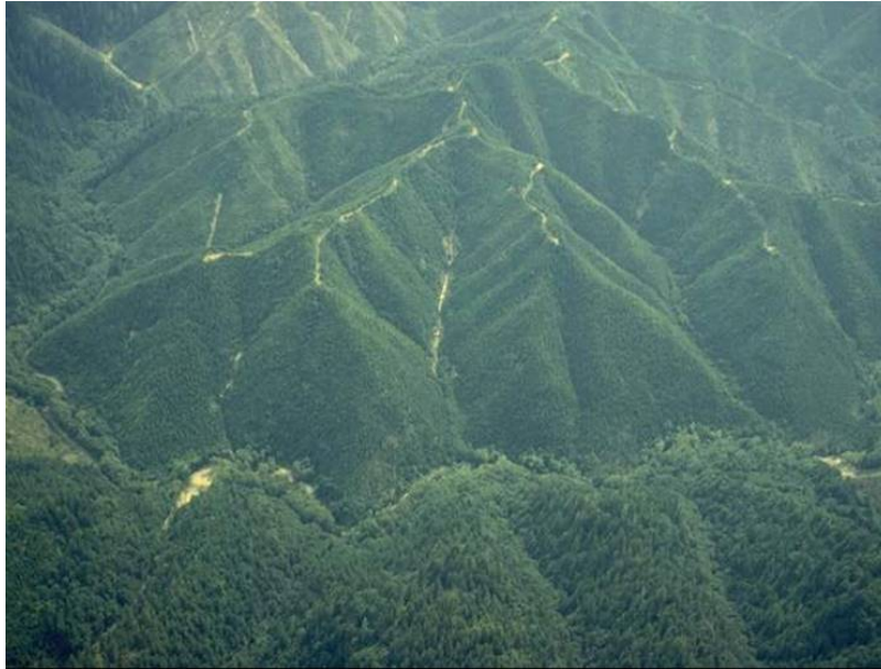
Figure 1: Debris Flow Catchments. This image shows characteristic debris flow dominated catchments in the Oregon Coast Range. The drainage network originates near the ridgecrests at colluvial hollows, where sediment accumulates over time. Evacuation of accumulated sediment and debris by shallow landsliding during large storm events trigger debris flows, which traverse the network and scour to bedrock.
