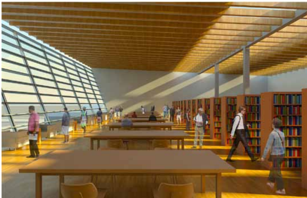
Figure 81: A library reading room. Notice the shading devices on the exterior of the windows as well as the way the structure acts as shading for skylights (Yaman Tezcan).
