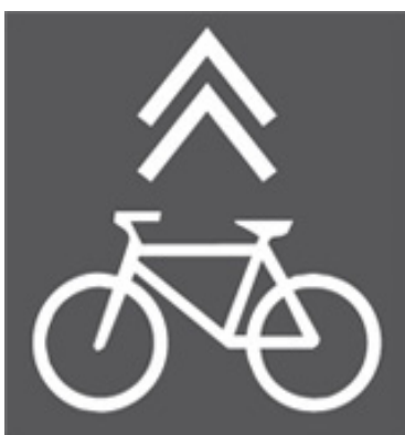
Figure 5: Sharrow designs include a bike with a double chevron in varying arrangements.
