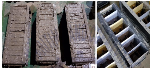
(b) Molds and removing plates before removing
