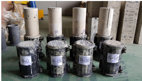
Fig. 2-9 Three steps for applying accumulated dead load on the specimen of splitting tensile tests
