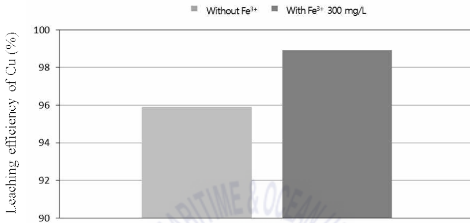
Fig. 16 Leaching efficiency of Cu with variation of Fe 3+ concentration
