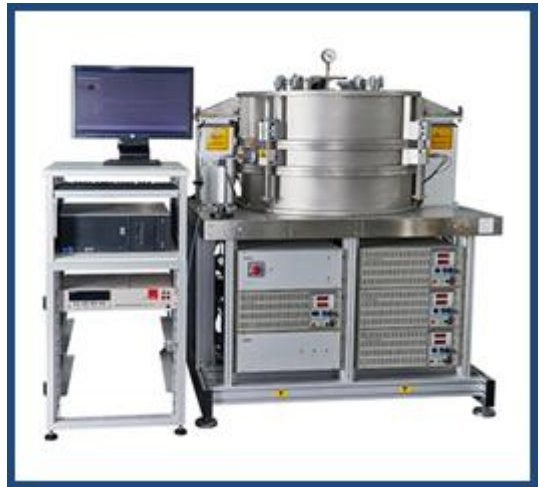
Fig. 2 Thermal measurement equipments(needle probe, guarded hot plate method)
