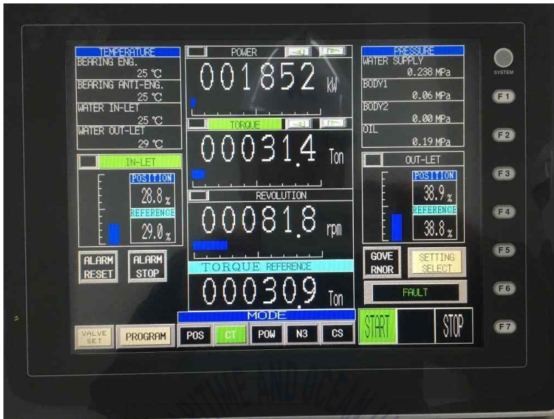
Fig. 4.8 Dynamometer control monitor (25% load)
