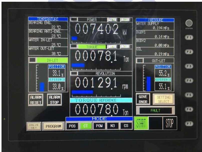
Fig. 4.11 Dynamometer control monitor (100% load)
