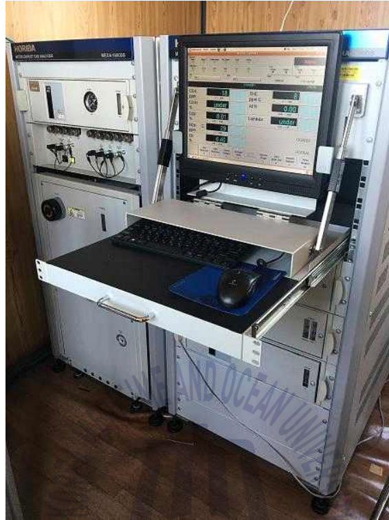
Fig. 3.11 Exhaust gas analysis system
