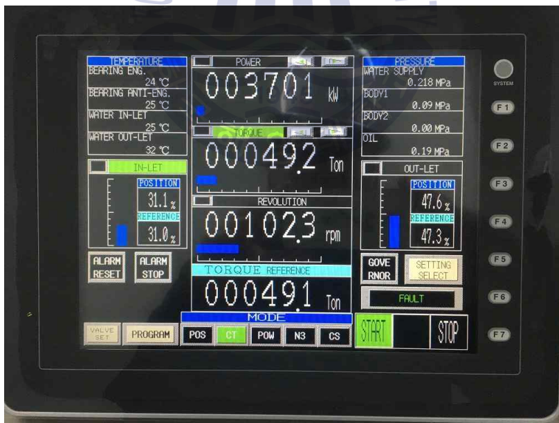
Fig. 4.9 Dynamometer control monitor (50% load)
