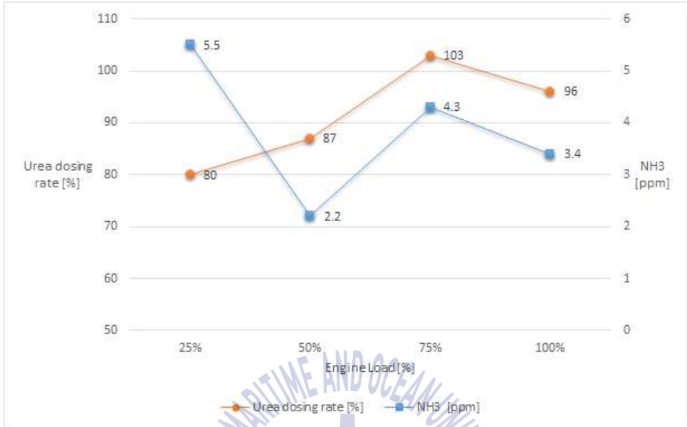
Fig. 4.15 Ammonia slip graph of SCR system
