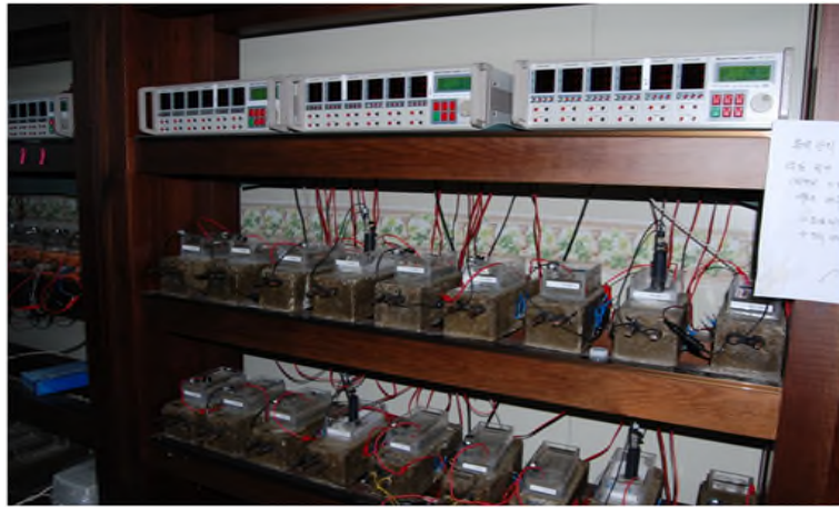
Figure 4.6 Picture of cathodic protection test on the beam type concrete specimens
