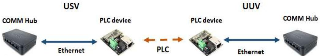
Fig. 4.6 Schematic diagram of USV-UUV communication
