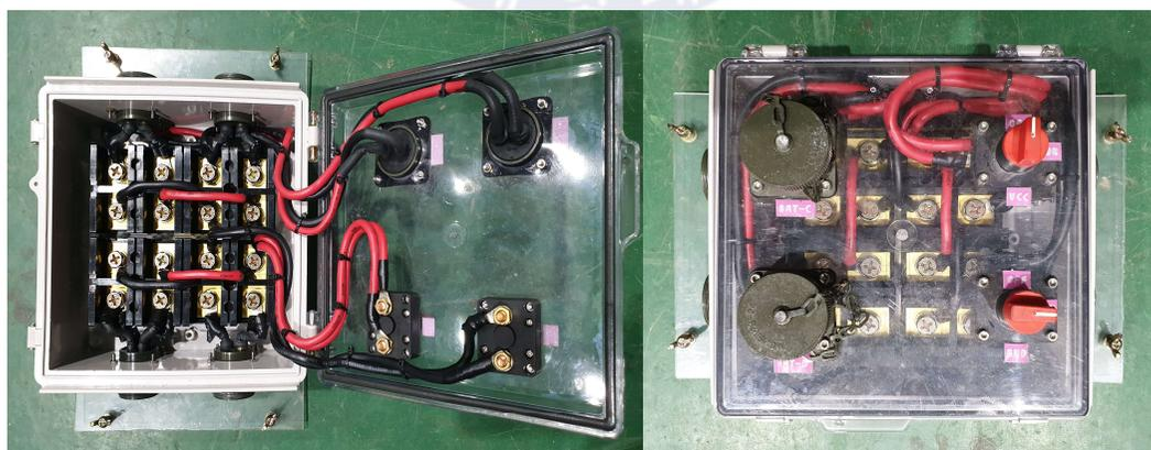
Fig. 3.2 Main power box of USV
