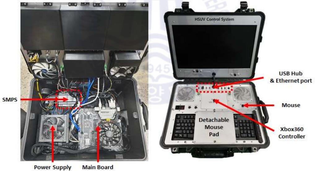
Fig. 3.16 Operating console for integrated platform
