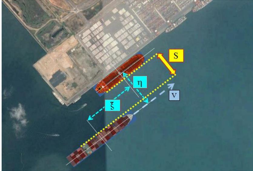
**Fig. 4.2** Diagram of passing ship and moored ship
