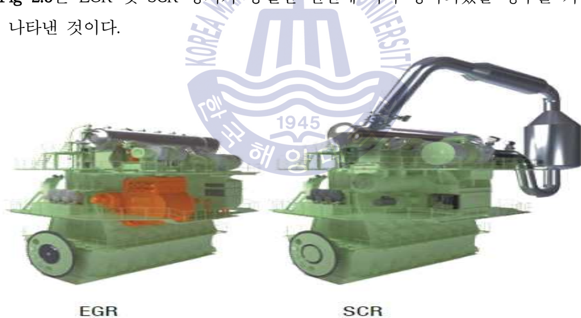
Fig. 2.5 Two-way approach for Tier III engine - EGR and SCR solutions [5]
