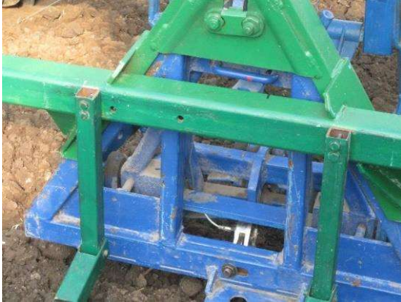
Figure 4. SA-type dynamometric automatic hitch with traction strain-gauge link.
