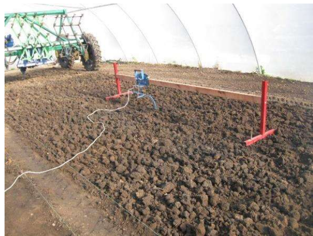
Figure 3. Automated field surface profile recorder.
