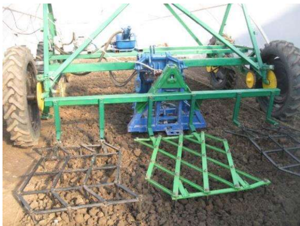
Figure 1. Harrowing unit based on gantry agricultural implement carrier.
