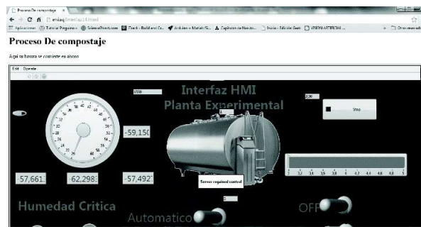
Figure 16. View of HMI control panel from a web navigator.
