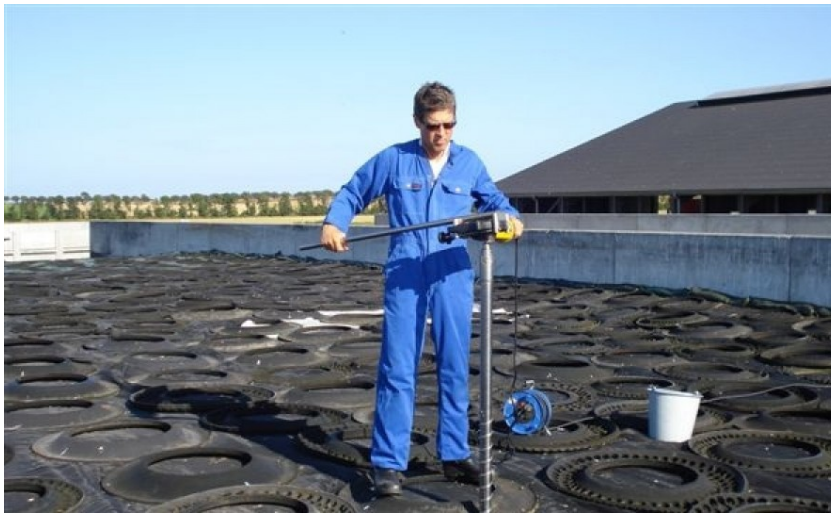
A silage auger may be used for sampling solid manure or deep litter heaps.
