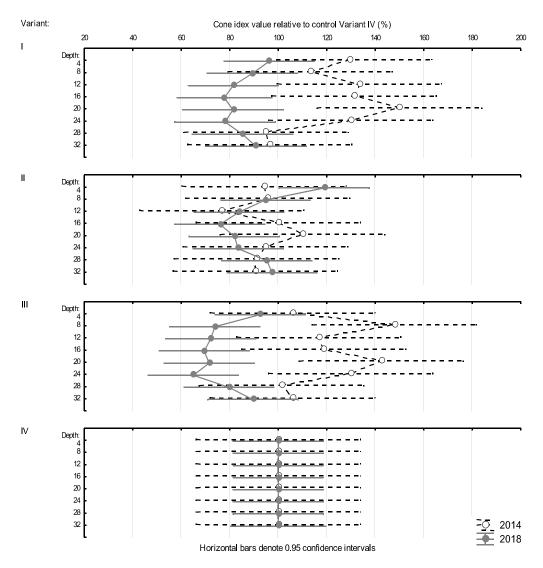
**Figure 4.** Graph comparing relative differences of cone index values to the depth up to 0.32 m for individual variants in spring 2014 and 2018 (Variants: I - FYM with Z'fix; II - FYM with Z'fix + NeoSol; III - FYM; IV - Control as 100%).
