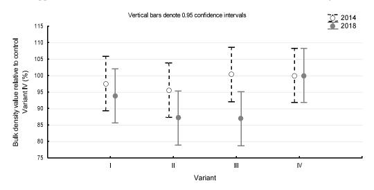
**Figure 3.** Graph of relative soil bulk density values from the depth of 0.05 to 0.10 m for individual variants in spring 2014 and 2018 (Variants: I – FYM with Z'fix; II – FYM with Z'fix + NeoSol; III – FYM; IV – Control as 100%).
