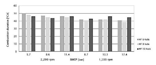
Figure 8. Combustion duration (°CA) at all engine loads, determined as crank angles between MFB 5% and MFB 90%.
