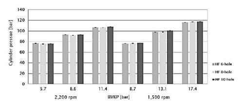
Figure 5. Maximum cylinder pressures at rated and intermediate speed with standard deviations.
