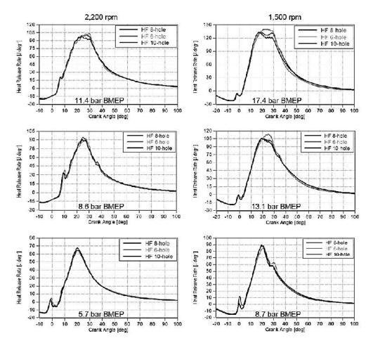
Figure 4. Heat release rates at rated and intermediate speeds.
