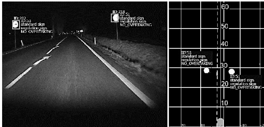
Figure 4. The screen view of two visualization filters of ADRF. (Left) Video widget with the filter of recognition all traffic signs. (Right) Coordinate graph for determining RD of the signs. Source: ADTF development environment.
