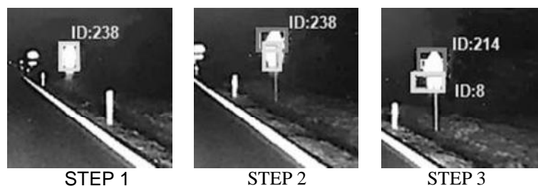
Figure 6. The problem in recognition of two traffic signs on a post is demonstrated in three steps. Source: Adopted from the ADTF development environment 1 .
