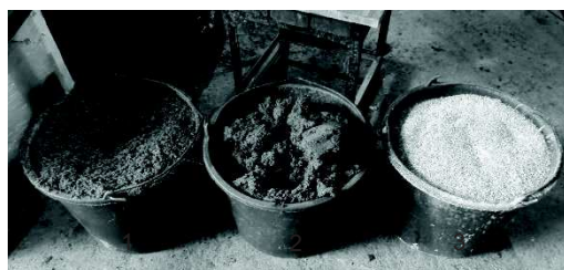
Figure 1. The components of the fermented mixture: 1 – the solid fraction of pig slurry coming from the screw separator; 2 – the solid fraction of pig slurry coming from the decanter centrifuge; 3 – grain mechanical cleaning waste.
