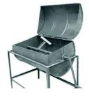
**Figure 3.** Prototype reactor with a temporary manual rotation system.
