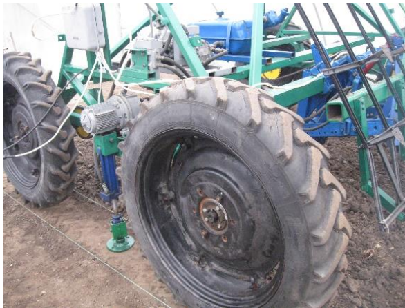
Figure 1. The agricultural gantry system used for experimental studies on the work of its pneumatic wheels.
