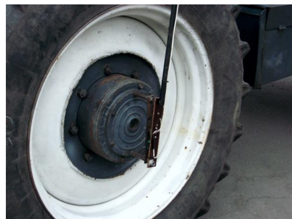
Figure 6. Wheel rpm pickup
