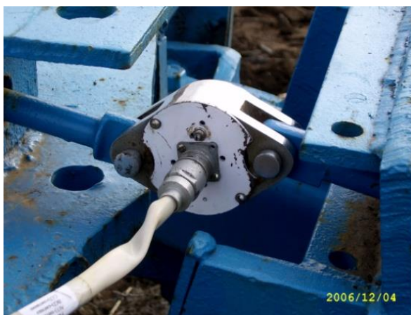
Figure 5. Draught strain-gauge link
