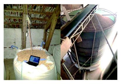
Figure 1. The storage of spelt grain in a FIBC bag (on the left) and in a tower silo with steel wire construction and textile liner (on the right).
