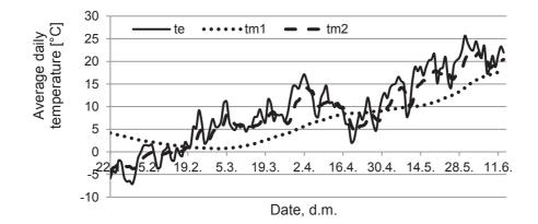
**Figure 2.** Comparison of the average daily outdoor temperature and average daily temperature in the spelt layer of both storage structures in 2017.
