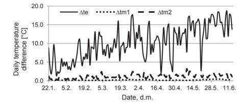
**Figure 3.** Comparison of the average daily outdoor temperature differences and average daily temperature differences in the spelt layer of both storage structures in 2017.
