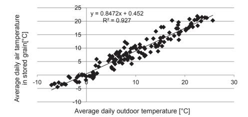
**Figure 5.** Comparison of the average daily outdoor temperature and average daily temperature in the spelt layer in the bag in 2017.
