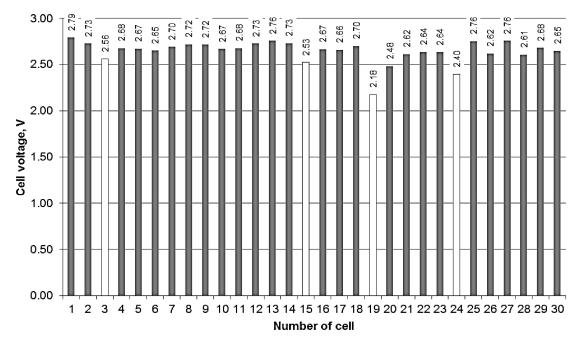
Figure 6. Average readings of the voltage measurements of the batteries under load.
