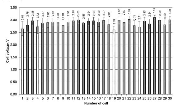
Figure 3. Average readings of the voltage measurements taken after the electric vehicle had covered a distance of 55 km.
