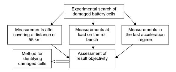
Figure 1. Sequential scheme of the experiment.
