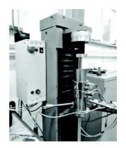
**Figure 2.** Testing stand for agglomeration process.
