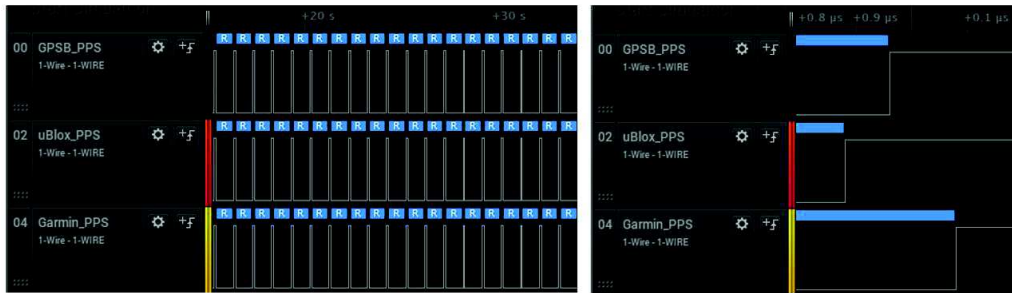
Figure 4. Screenshot of Saleae Logic logging software from the measurement of three PPS signals.
