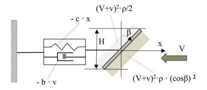
Figure 6. Model for obtaining renewable energy from fluid.
