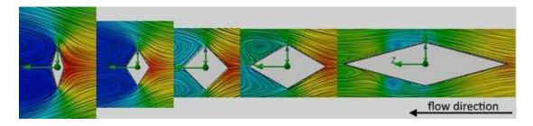
Figure 3. Stream lines and pressure distribution for the diamond body.
