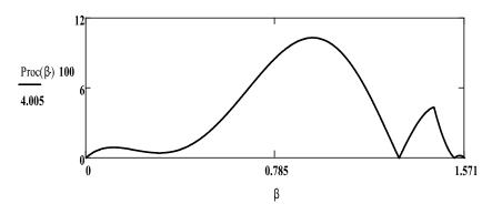
**Figure 4.**  $\beta$  radians against percentage difference. The accuracy of the approximate formula (8) for diamond plate when C = 0.5, expressed as a percentage. The mean value is about 4%.
