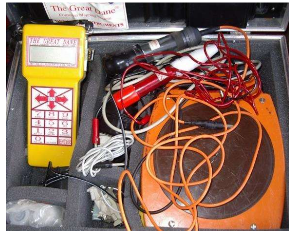
Figure 5. The Great Dane corrosion mapping system.
