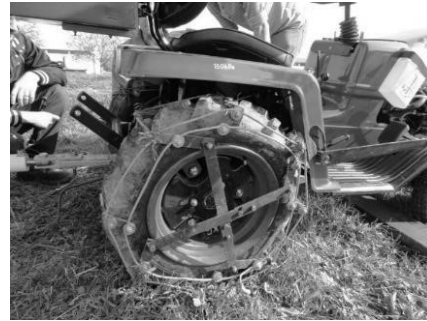
Figure 5. The test tractor Mini 070 type equipped with the special driving wheels.
