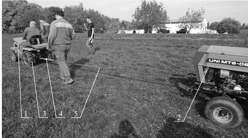
Figure 3. Measurement of drawbar pull of the tractor with special driving wheels: 1 – test tractor Mini 070 type; 2 – load tractor MT8-0652 type; 3 – special driving wheels; 4 – force sensor EMS 150 type; 5 – steel chain.
