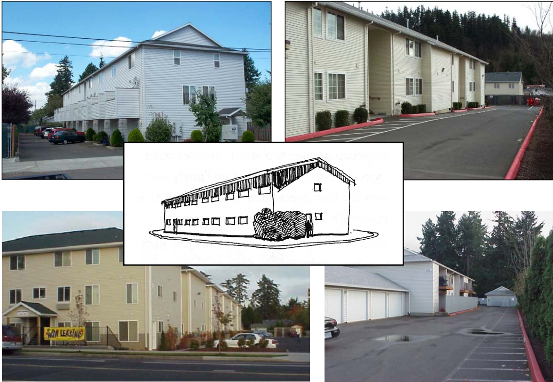
Examples of Outer East apartment developments , with typical barracks-like massing (similar to the inset image from Building Blocks for Outer Southeast Neighborhoods intended to highlight what should be avoided in the design of multidwelling projects). The narrow, deep lots of Outer East Portland tend to lend themselves to such arrangements.
