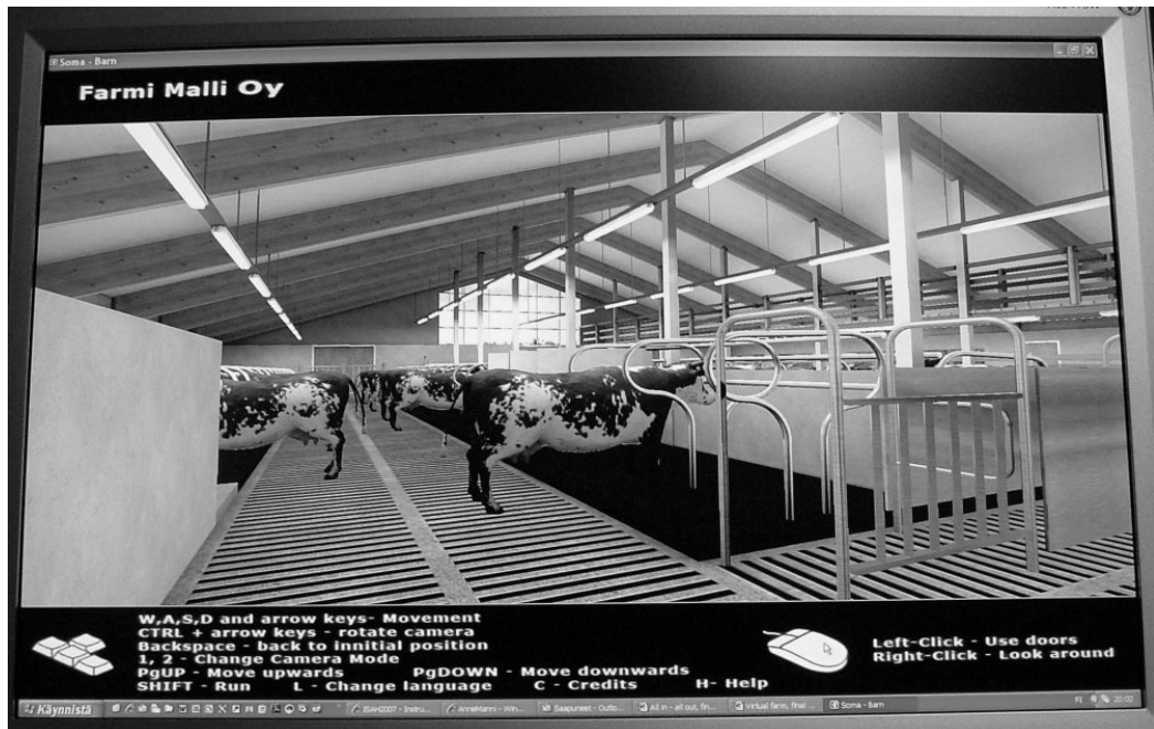
Figure 1. The Farm Designer is an internet based program designed to create 3D models of farms. It is possible to move freely inside and outside of the building and look at details. The 3D farm is the first step towards the Virtual Farm Project. Once finished, it will feature virtual animals that look and move in an authentic manner and react to the changes in the environment.
