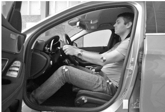
Figure 2. Test subject in the measuring vehicle with hands in the optimal position L9-R3.
