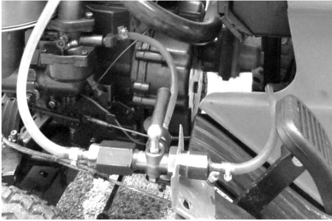
Figure 7. Three-way valve set to flow from the measuring tank.
