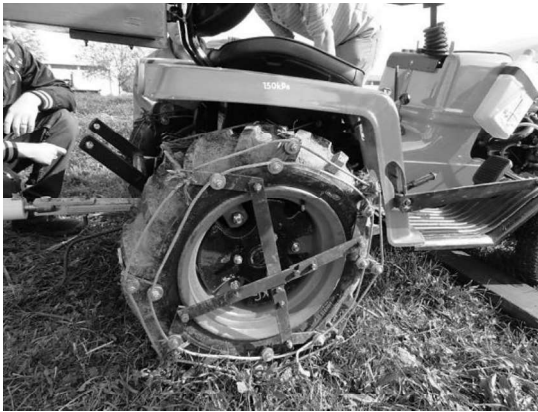
Figure 4. Spikes device on tractor wheel tyres TS – 02 type with 8 active spikes.
