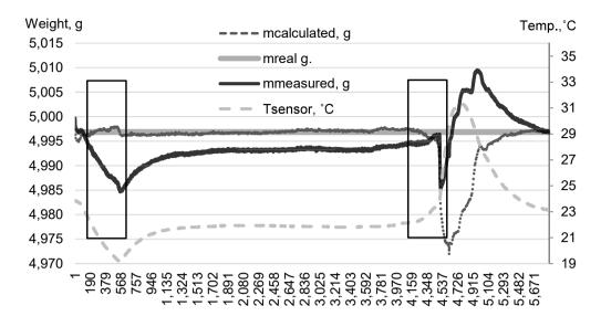
Figure 2. LSM reading stability experiment (impact of temperature test result).
