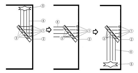
**Figure 1.** Principle of the automatically light panel: 1 - reflectors or sunlight; 2 - light panel body with rotating mechanism; 3 - light permeable triangles; 4 - light beams; 5 - lighting center. Please refer to the reference if this is not your own drawing.
