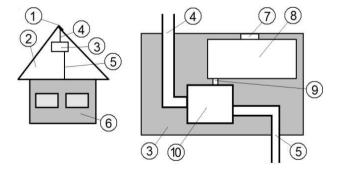
**Figure 4.** Distribution system: 1 – Sprayers; 2 – Roof; 3 – Tank; 4 – Mixed piping; 5 – Water supply system; 6 – Greenhouse; 7 – refilling opening; 8 – Integrated refilling tank; 9 – Dispenser; 10 – Mixing chamber.
