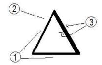
**Figure 2.** Principle of the light permeable triangle: 1 – light permeable sides; 2 – light permeable triangle; 3 – reflective sides.
