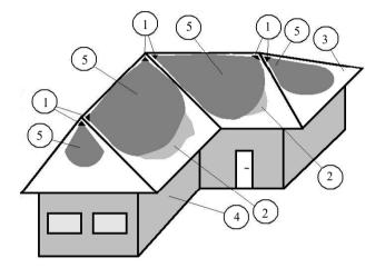
**Figure 3.** Applicator of inhibitors for protection of roofing: 1 – Sprayers; 2 – Plants of the order Porellales; 3 – Roof; 4 – Greenhouse; 5 – A copper sulphate mixture.
